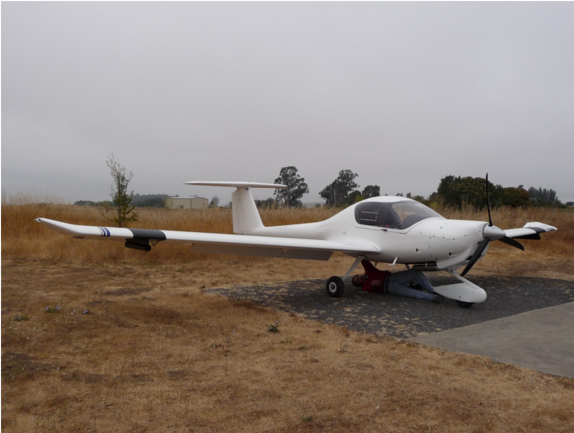
Figure 8 - Team Aerochia's Diamond DA20-A1 fitted with a bio-diesel boost engine
